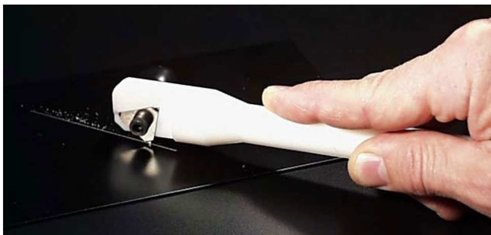
Fig. 3 Applying the scribed line / Ritsens anbringande
