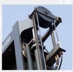
The DCF80-100 has considerably fewer hoses over the mast compared to conventional machines (2 hydraulic hoses and 1 electrical cable). This provides high functional reliability.
