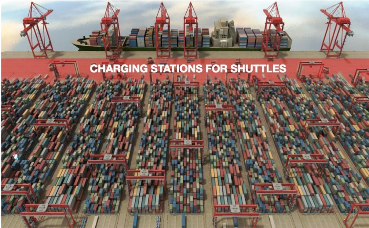
*Fast charging stations can be installed along the shuttle working route in order to utilize idle time for charging.*
