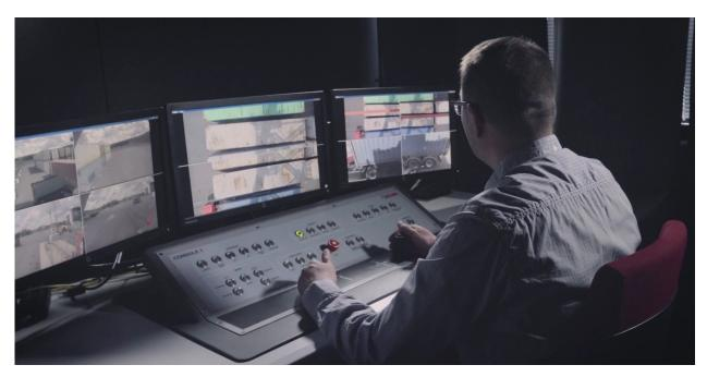
The most significant cost savings from automation are due to the drastically smaller number of operators required. Typically, a single operator can handle two to three AutoRTGs remotely, and in quiet periods even up to six machines.
