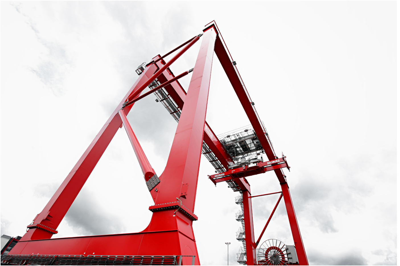
Figure A.3 Automated stacking crane (ASC)
